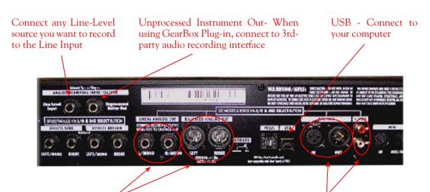
Analog Line Outs, Use either Unbalanced (1/4 -inch) jacks or Balanced (XLR) jacks to connect to your powered speakers or mixer
