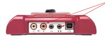
Connect a 1/8-inch stereo cord to the Headphone Out, or use the Stereo RCA Line outputs with an adapter.
