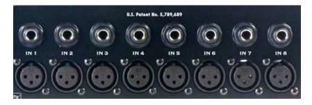
8 unbalanced line level inputs are available for recording line level sources, such as a keyboard, stereo receiver, the line out from a mixing console, etc. Connect to line level inputs using 1/4-inch TS audio cables.
