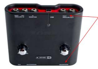
Connect the mono 1/4-inch Analog Line Outputs.
