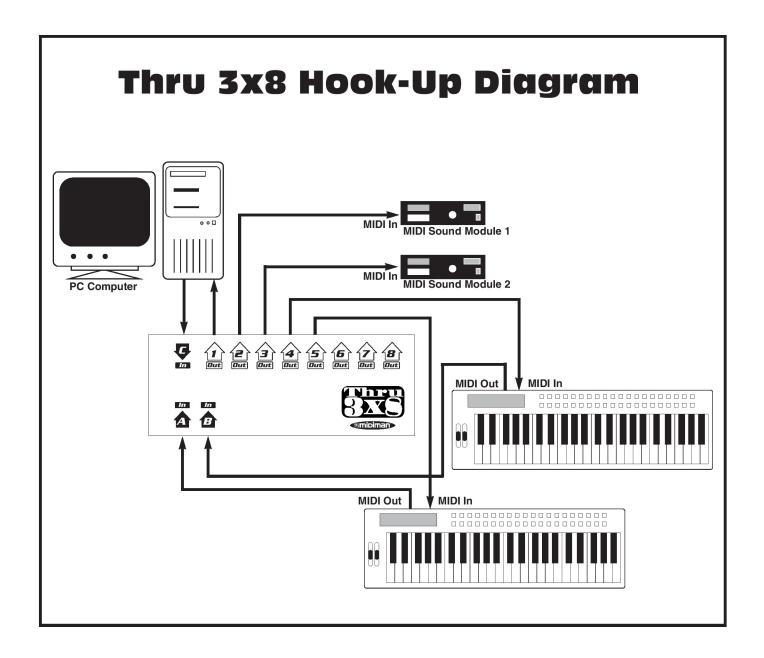
Also, any MIDI signals received at any of the Thru 3x8's MIDI ins are simultaneously sent out all of selected MIDI outs. So the Thru 3x8 can be used to eliminate any "MIDI delay" you may be experiencing because of daisy chaining several MIDI devices together.
