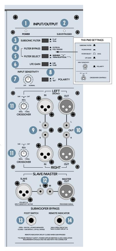
Frequencies below the crossover frequency are sent to the subwoofer, and frequencies above the crossover frequency are sent to the LEFT and RIGHT OUTputs, which are connected to the main/satellite speakers.
