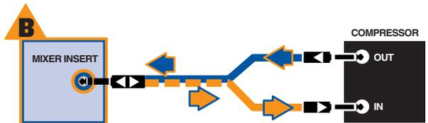
Figure B is a closeup of Figure A. The two colors represent the input and output traveling the length of the "Y" cable. The dotted line represents the two signals travelling alongside one another.
