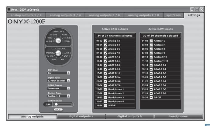
When 176.4/192 kHz sample rate is selected, 8 inputs and 8 outputs are available. Again, you can modify the default settings by deselecting one or more pairs of audio streams and selecting other pairs. As soon as all of the available audio streams are used up, the remaining inputs and outputs are "greyed" out.
