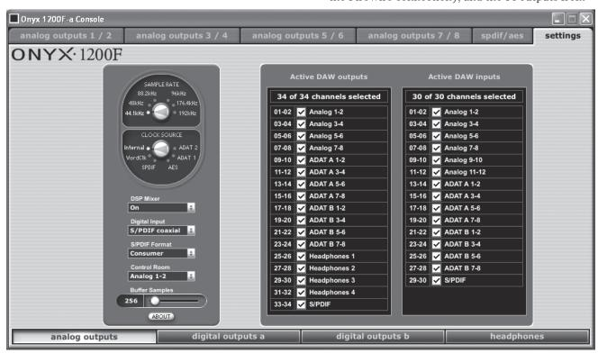
the DAW back to the Onyx 1200F outputs. All the Output tabs are unavailable and the matrix mixer cannot be adjusted.
