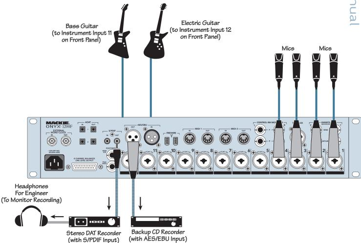
This illustrates a simple direct to 2-track recording setup. You can configure the Onyx 1200F beforehand with the desired sampling rate, with the inputs routed to the S/PDIF output. The AES/EBU output on the Onyx 1200F carries the same signal as the S/PDIF out, and is connected to the AES/EBU input on a stereo CD recorder for backup.
