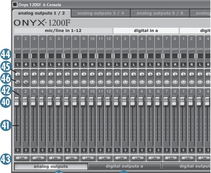
A LINK button [43] allows you to link the faders of adjacent channels (odd/even pair) so they move together when using them as a stereo pair.
