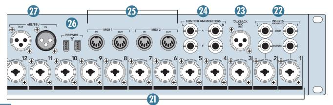
The twelve mic/line inputs, two S/PDIF or AES inputs, eight digital A, and eight digital B inputs are routed directly to the software application via the FireWire connection. These streams are not affected by the DSP Mixer in the Onyx 1200F Console (see the Figure on page 9).
