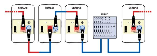
Multiple SRM450 "Daisy-Chaining" using signal pass-thru connection
