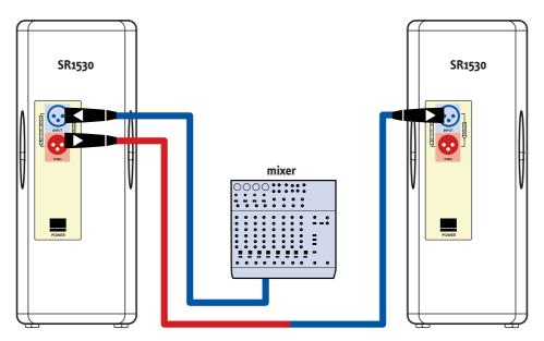
Two-speaker mono hook-up using signal pass-thru connection
