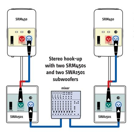
Connect the Main Outs on your mixer to the inputs of your SWA1501 Subwoofers, then from the Hi-Pass Thru connector of the subwoofers to the SRM450 inputs.
