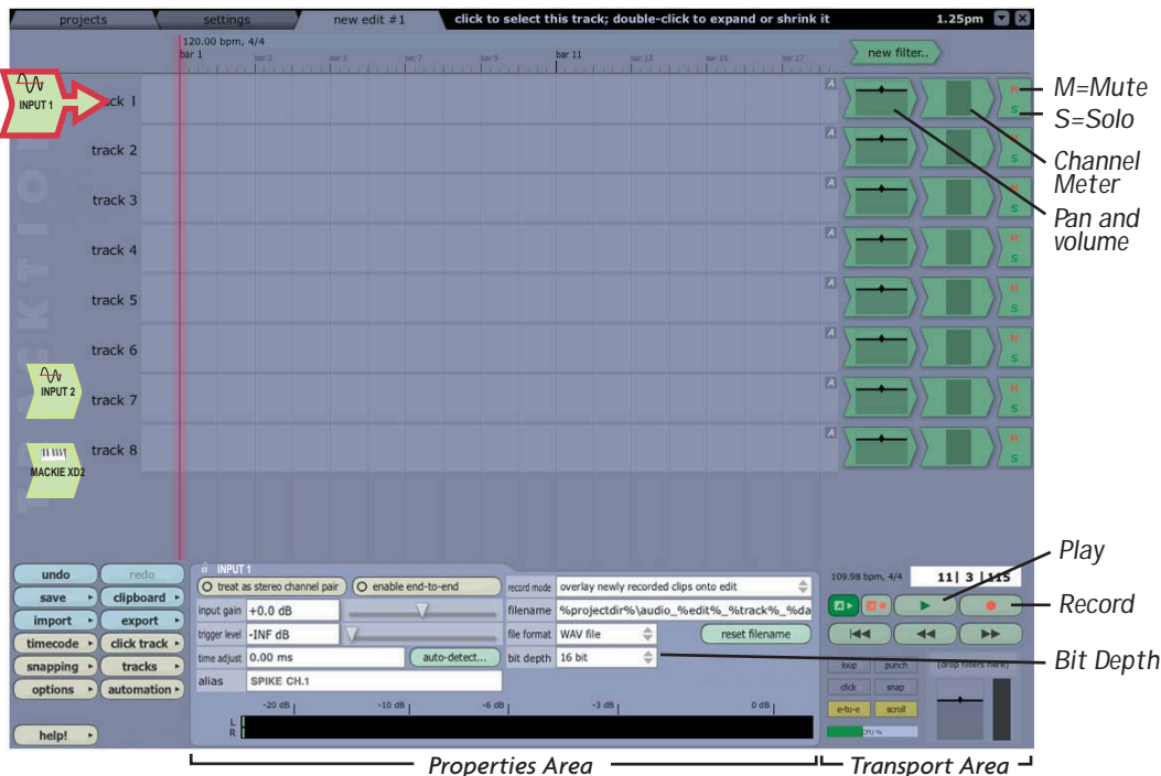
Tracktion Edit Screen (with connected Input 1 Icon, shown larger than real size)
