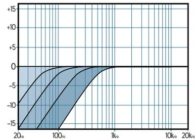
The HPF (high pass filter) switch, often referred to as a low cut filter, cuts bass frequencies at a rate of 12dB per octave below a swept-select point, ranging from 30Hz–800Hz. Using HPF will clean out the “mud” in your mix, can help reduce the possibility of feedback in live situations, and help to conserve amplifier power.
