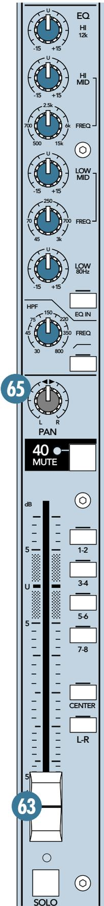
LEFT/RIGHT mix **67**. If you want to create a Subgroup of certain Channels, engage one of the numbered switches instead of the L-R, and the signals from those Channels are sent to the appropriate Subgroup Fader **95**. From there, the Subgroups can be sent back to the main LEFT/RIGHT mix **87**, allowing you to use the Subgroup Faders as a master control for those Channels.
