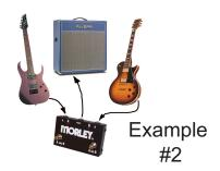
GROUND LOOP NOISE? Hooking two amps together via an ABY box can sometimes create a LOOP ANTENNA which causes hum (also known as Ground Loop Hum, 60Hz Hum or 60 Cycle Hum, 50Hz in Europe). This is not caused by the ABY but by the connection of two amp grounds via the ABY. If this does occur, it can be easily corrected. Visit www.ebtechaudio.com for information on eliminating Ground Loop Hum & Noise with our Hum X or outside North America. the Hum Eliminator.
