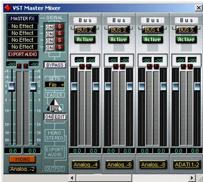
Figure 6-3: Use the output buttons at the bottom of each channel strip to assign MOTU 828 outputs to busses. You can then assign channels in the Monitor window to each bus as desired.
