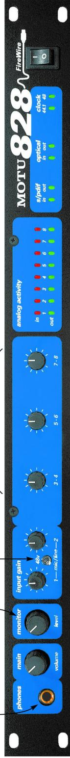
These two trim knobs provide up to 40dB of gain for inputs 1 and 2. Because inputs 1 and 2 also have microphone pre-amps, you can plug just about anything into them: a microphone, a guitar, an synth — your name it.
