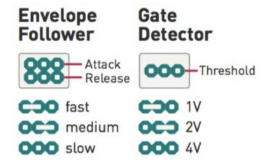
The last setting, corresponding to the longest time or higher voltge, is obtained by removing the jumper.
