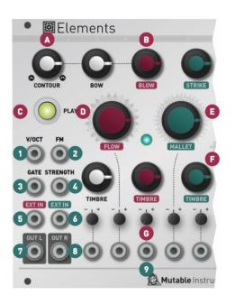
**A**. Bow/Blow envelope **CONTOUR**. A simple envelope is applied to the sound generated by the **BOW** and **BLOW** exciters. This knob interpolates between several preset shapes for this envelope: short AD envelopes getting longer and slower, morphing into slower ADSR envelopes, fading into faster AR envelopes.
