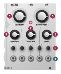
The main frequency of the sound is controlled by the **COARSE / FINE** knobs, combined with the **V/OCT** and **FM** CV inputs.
