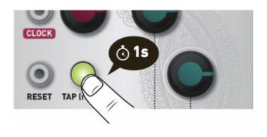
Unplug all CV inputs and hold the **TAP/reset** button for half a second to adjust Grids' options. The switch stays illuminated. Hold the button again for half a second when you are done.
