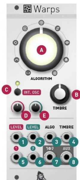
**A. Modulation algorithm.** This knob selects which signal processing operation is performed on the carrier and modulator. The algorithms are described in further details in the next section.
