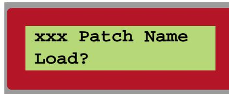
3. Select the desired patch to load with the **ROTARY DIAL** or with the left/right **NAVIGATOR** buttons and load the patch to the **SLOT** by pressing the **PATCH/LOAD** button again. To switch between entire patch banks, you can also use the up/down **NAVIGATOR** buttons.
