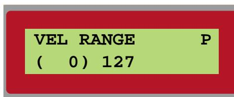
Set the lowest and highest velocity values. The patch will only sound when it receives velocity within this range. If you want to use Nord Modular to switch between two or more patches that are set to receive on the same MIDI channel (velocity switching), select two SLOTS, set them to the same MIDI channel, make sure that the Keyboard Mode is set to Selected Slots, and set the velocity range individually for the patches.
