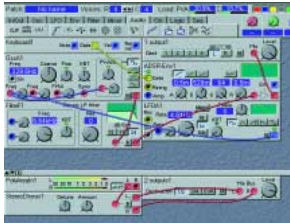
This is a patch that uses both the Poly and Common Voice area of the patch. The requested and current number of voices is 4. Schematically, the patch will require the PVA Load x 4 voices + 1 x the CVA Load. You could also see it this way:
