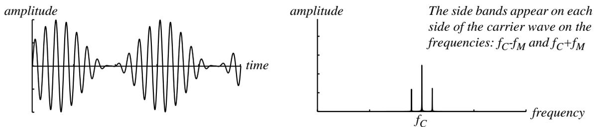
**Fig 3. Amplitude Modulation**
