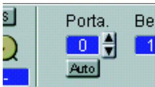
The portamento has two modes: Normal and Auto. In the Normal mode the portamento is always active, in the Auto mode you activate the portamento by playing legato. With the up and down buttons you set the time it should take to reach the new note.
