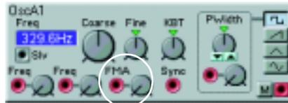
A signal routed to an FM input on a module affects the pitch by modulating it linearly in the **frequency** scale (see figure below). The figure shows an A4 note being pitch modulated by a symmetric bipolar signal.
