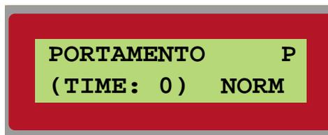
The portamento has two modes: Normal and Auto. In the Normal mode the portamento is always active, in the Auto mode you activate the portamento by playing legato. This portamento function is available only if a patch is set to 1 voice, i.e. monophonic. The Portamento function is always active on any keyboard tracking oscillators used in the Common Voice Area, since this is a monophonic area. A portamento Time setting of '0' is the same as portamento 'off'.
