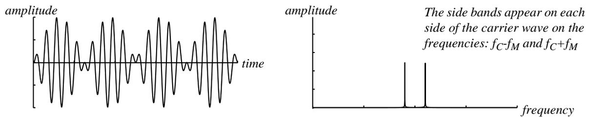
**Fig 6. Ring Modulation**
