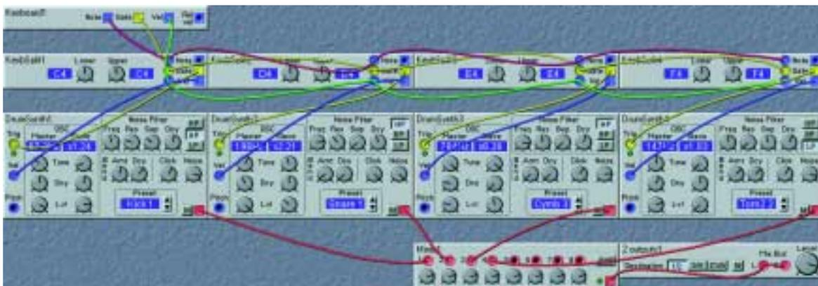
First, a Keyboard Voice module is used to be able to patch Note, Gate and Velocity signals to the other modules in the patch. To filter out four separate keys to trig each of the four Drum synth modules, we use four Keyboard Split modules. We make a serial connection of the Note, Gate and Velocity cables from the Keyboard Voice module to the corresponding inputs of the four Keyboard Split modules.
