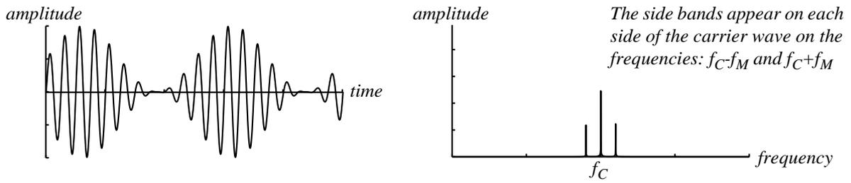
**Fig 3. Amplitude Modulation**
