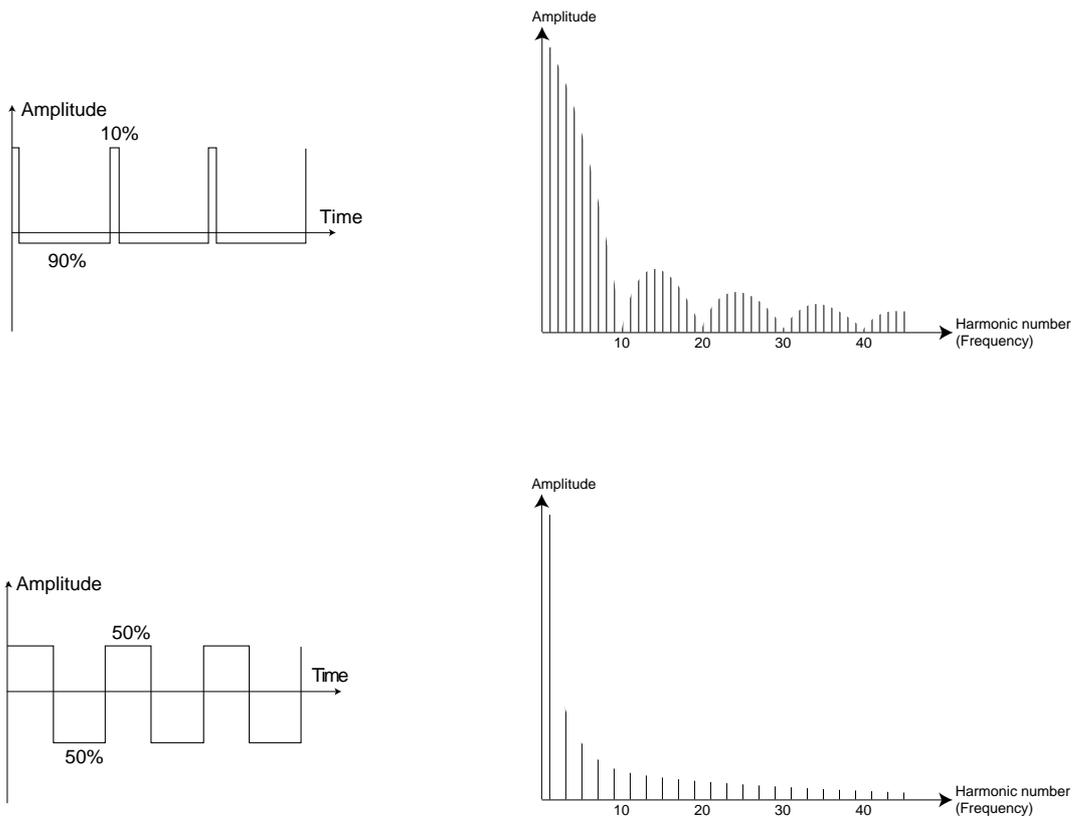
In the first example, the jump happens 5% in from the beginning of the period. This is referred to as a pulse wave with a 5% *pulse width* (sometimes called *duty cycle*). The second wave has a pulse width of 10%. The third wave has a pulse width of 50%. The third wave is a special case of the pulse wave, called a *square wave*, and this has one peculiarity, it only contains odd number harmonics, which gives it a “hollow” quality.
