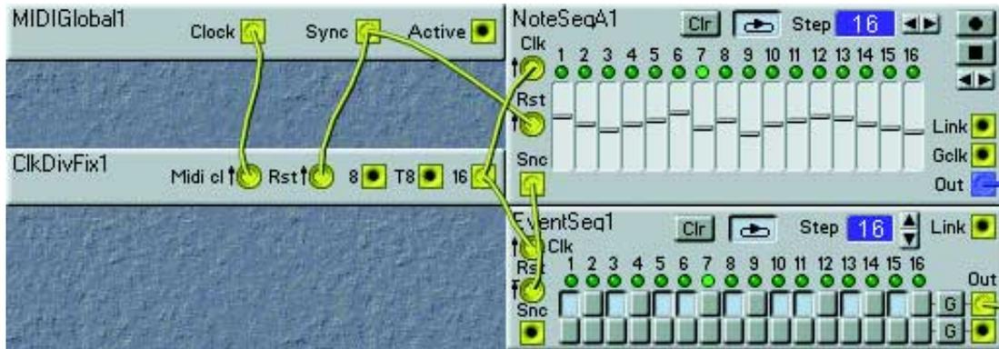
In this example the Rst signal to the sequencers is taken from the MIDI Global module to the Note Sequencer, then transmitted from the Snc output to the Event Sequencer. The Event Sequencer in this example has the loop mode turned on. This doesn't matter in this setup since the Rst signal received from the Note Sequencer Snc output will reset it to step 1 after each loop of the Note Sequencer.
