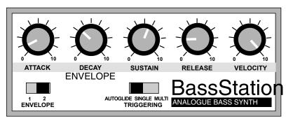
switch below Pulse Width and the Filter Mod switch in the Filter section. Of course, if neither of these is switched to Env 2, you will hear no change when you alter the settings of Envelope 2. Switch one or the other to Env 2 to hear the changes you are making.
