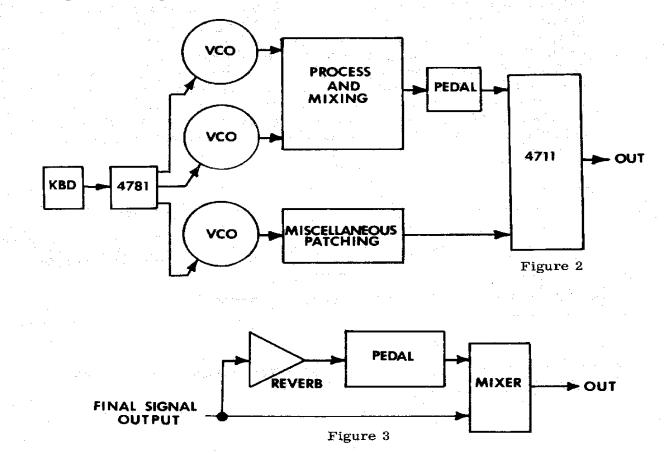
As the pedal has no capacitive coupling, control voltages can be processed without fear of loosing DC levels or low frequency waveforms. For use with control voltages, your other set of patch cords ( with pin plug connectors) will be used. Patch configuration is similar to audio use, with the control voltage source being fed to the pedal input, and the pedal output being fed to the module to be controlled.
