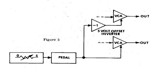
Another interesting type of pedal control can be obtained by using an audio cord to apply a higher frequency signal to the input of the pedal, and using a control voltage co d to apply the pedal output to the control input of a module. Try this with a VCO feeding another VCO or a VCF.
