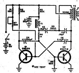
Fig. 1. The circula is not as simple as it looks. Besides a multivibrator, there is also a blocking oscillator in there. All components are part of one time constant or another, so changing the value of one will alter the final sounds. Note the speaker damping (R8) that keeps speaker acoustic loading from altering the oscillator.
