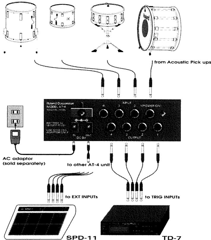
\* **INPUT 1** also functions as the power switch, so be sure that it is connected when you wish to use the AT-4. (A stereo cable cannot be used.)
