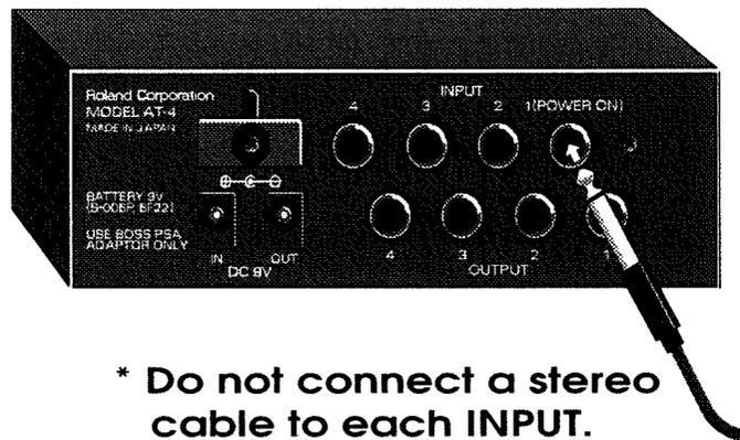
**\* Do not connect a stereo cable to each INPUT.**
