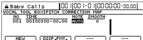
In the Correction Event Map screen, you can input the time at which you want the pitch correction to start as well as the pitch.
