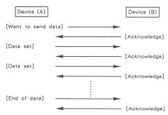
Device (A) requests and receives data from device (B).
