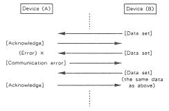
Device (B) rejects the data re-transmitied, and completes data transfer.
