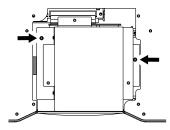
Replace the cover with the positions of the (A) and (B) sections of the cover are reversed relative to their positions prior to the cover's removal.
