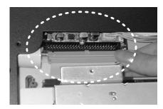
Position the CDI-BR-1 as shown in the figure so that the CDI-BR-1's and BR-1180's attachment holes are aligned.
