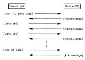
Device (A) requests and receives data from device (B).
