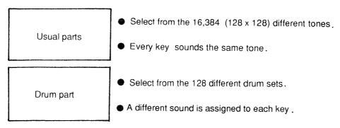
Roland drum machines and percussion sound modules all send and receive MIDI data on MIDI channel 10 as a standard. Likewise, GS sound sources power up with MIDI channel 10 as the default channel for drum parts.
