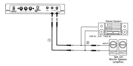
① Plug the cables into the CM-500's Audio Outs.
