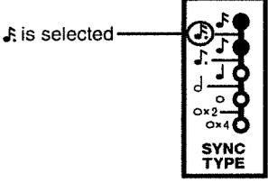
\* [EXIT] + [SYNC TYPE] selects a triplet; the LEDs will be lit in reverse.
