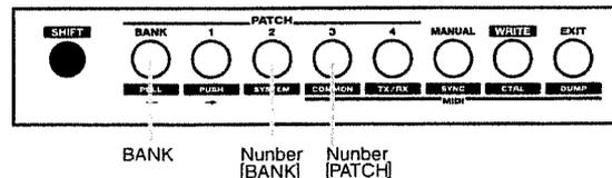
Press the [BANK] button, then press the [2] button. This selects Bank 2. Next, press the [3] button. This selects Patch No. 3 in BANK 2, "SLICER + PAN."
