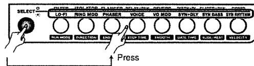
When the [SELECT] button is extinguished, you can select the effects appearing in the upper row of the panel (e.g., FILTER or ISOLATOR)
