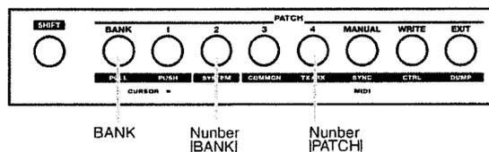
Press the [BANK] button, then press the [4] button. This selects Bank 4. Next, press the [2] button. Patch No. 2 of BANK 4, "SYN + DLY" is now selected.
