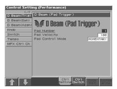
**3.** Press [5 (Ctrl Setting)] – [6 (Ctrl Switch)] to select the parameter. [5(Ctrl Setting)]: Controller-related settings, Settings for the entire performance
