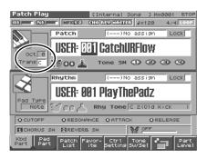
5. Either turn the VALUE dial or use [INC]/[DEC] to adjust the Transpose setting (G-F#: -5-+6 semitones).
