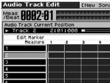
Use the cursor buttons (up/down) to select the desired track. You can specify the location at which the sample will be inserted using the following units.
