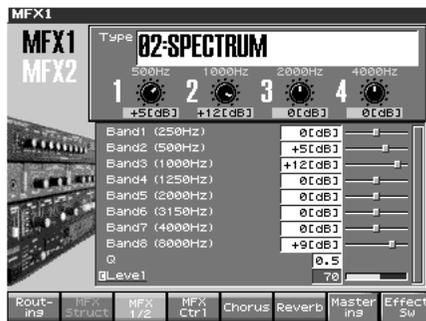
1. Press [EFFECTS] to access the Routing screen, and change MFX-1 to “2: SPECTRUM.”
