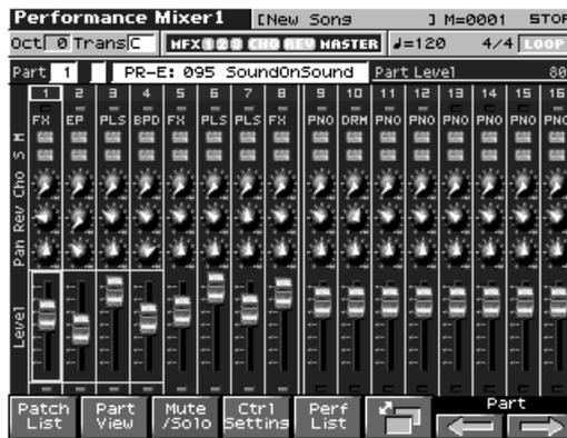
\* To adjust the volume balance between the keyboard and pads in Patch mode, access the Patch screen and press [F3 (Part Level)] to access the "Part Level" screen.
