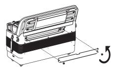
(5) Remove the cover from the FR-7b/FR-5b's battery compartment.
