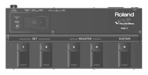
Use the **SET** switches (1 and 2) to select Sets. The 1 switch allows you to select the preceding Set (e.g. Set 18 if you are currently using Set 19), while the 2 switch is used to select the next Set (e.g. 20 if you are currently using Set 19).
