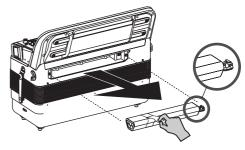
The battery is connected to the FR-7b/FR-5b by means of a cable. You need to disconnect the cable from the battery by pressing the clip on the connector before fully removing the battery.
