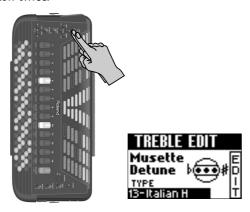
(2) Use the <u>DATA/ENTER</u> knob to select the a different tuning for the Treble reeds.
