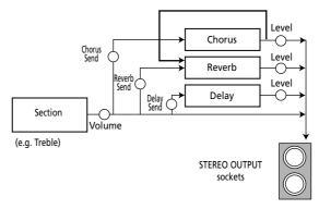
■ Chr Dly (0~127)—This parameter sets the amount of chorus sound that is sent to the Delay processor. Higher values result in more sound being sent. The value "127" effectively allows you to connect the Chorus and Delay effects in series (Chorus before Delay). If you do not want the chorus signal to be processed by the Delay effect, set this value to "0".
