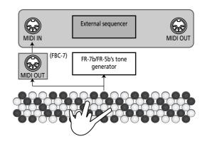
If the FR-7b/FR-5b is used as tone generator for an external sequencer, you must connect the sequencer's MIDI OUT socket to the FBC-7's MIDI IN port (because MIDI data always go from OUT to IN).
