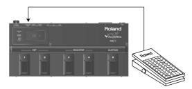
The expression pedal can be used to fade the Orchestra part in and out, which is probably most effective in DUAL mode (see p. 26). When the expression pedal is all the way up (heel down), the Orchestra part does not sound. Press the expression pedal down (toe down) to increase the Orchestra section's volume.
