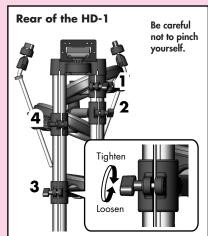
1. Attach the snare pad to the rod.
