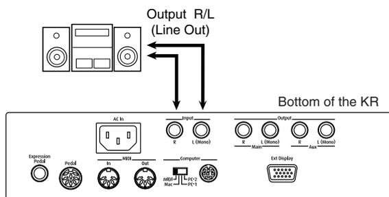
1. Turn the volume all the way down on the KR and on the device you're about to connect.
