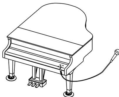
1. Connect a microphone (sold separately) to the Mic In jack on the lower-right area of the instrument.
