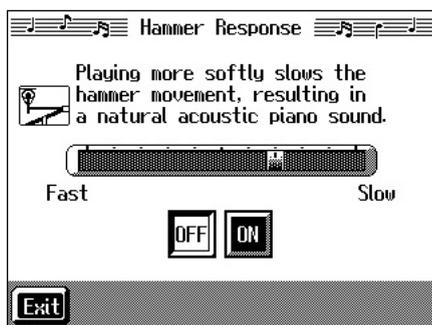
Touch <ON> to turn the Hammer Response function on.
