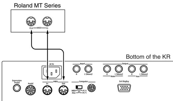
\* When the KR is connected to a MIDI sequencer, set it to Local OFF. Refer to "Disconnecting the Keyboard from the Internal Sound Generator (Local On/Off)" (p. 174).
