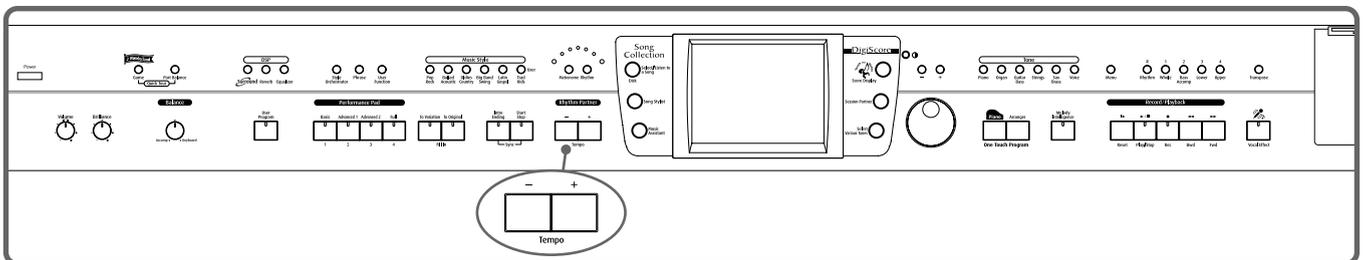
When the Basic screen is displayed, you can use the Tempo [-] [+] buttons or the [-] [+] buttons and the dial to change the tempo. The tempo is indicated on the upper left of the screen.
