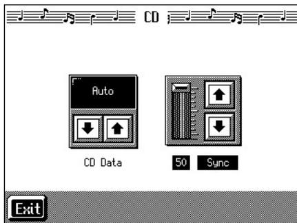
3. Touch the <Sync> slider to adjust the timing of the piano sound.
