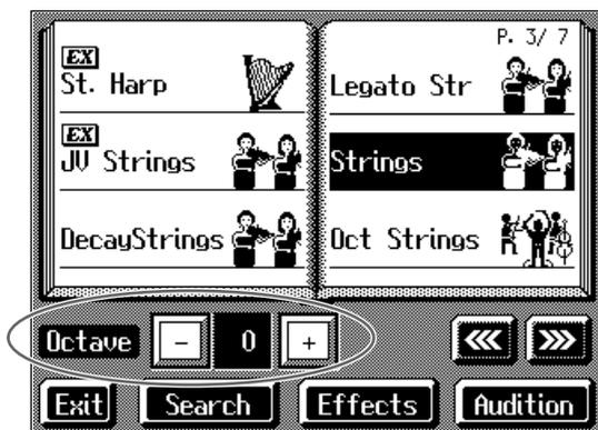
4. Touch Octave <-> or <+> in the lower part of the screen to adjust the pitch of the sound.
