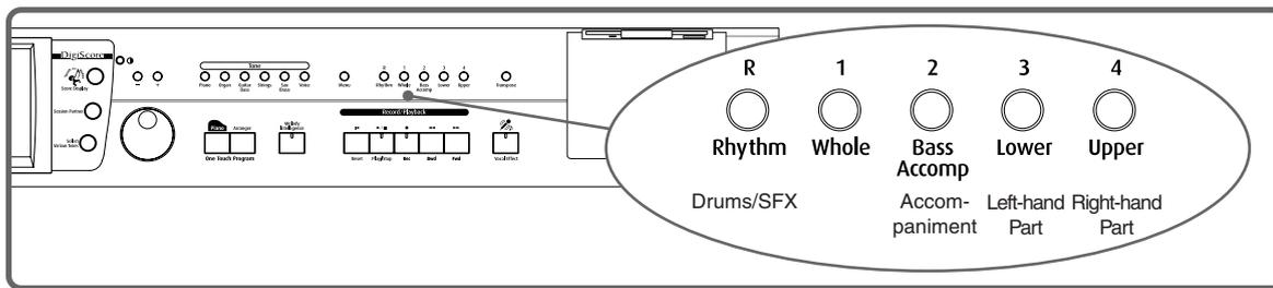
By using these Track buttons, you can eliminate the sound of specific parts. This is referred to as “muting.”
