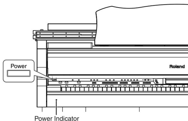
**To turn the power off, turn the [Volume] knob all the way to the left, and press the [Power] switch.**
