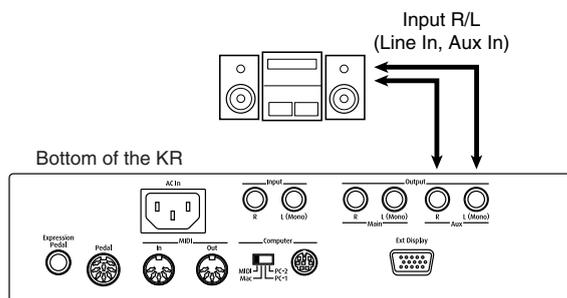
1. Turn the volume all the way down on the KR and on the device you're about to connect.
