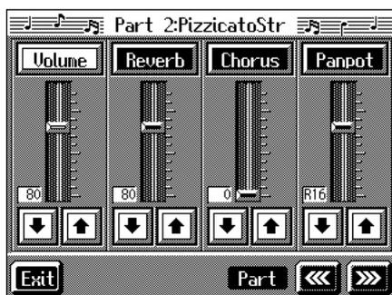
You can change the Tone for the selected Part by pressing a Tone button while this screen is displayed. When selecting Part 10 or 11, you can touch <Drum Set> to select the drum set or effect sound.
