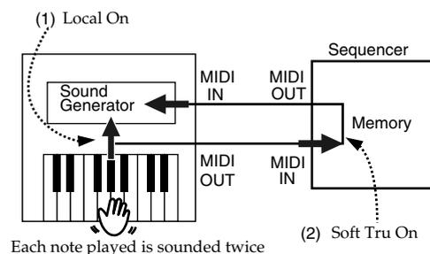
**Local On:** The keyboard and internal sound generator are connected.
