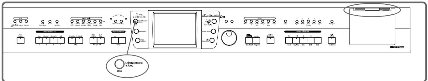
First make sure that the protect tab of the floppy disk is in the "Write (write enable)" position.
