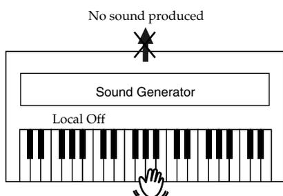
→ When connecting a unit in the Roland MT series, you don't need to switch off Local Control. MT units transmit Local Off messages when their power is switched on. If you first switch on the KR, then the MT-series device, Local Control is automatically switched off on the KR.
