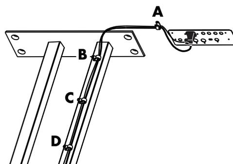
1. Connect the supplied power cord to the AC inlet jack.
