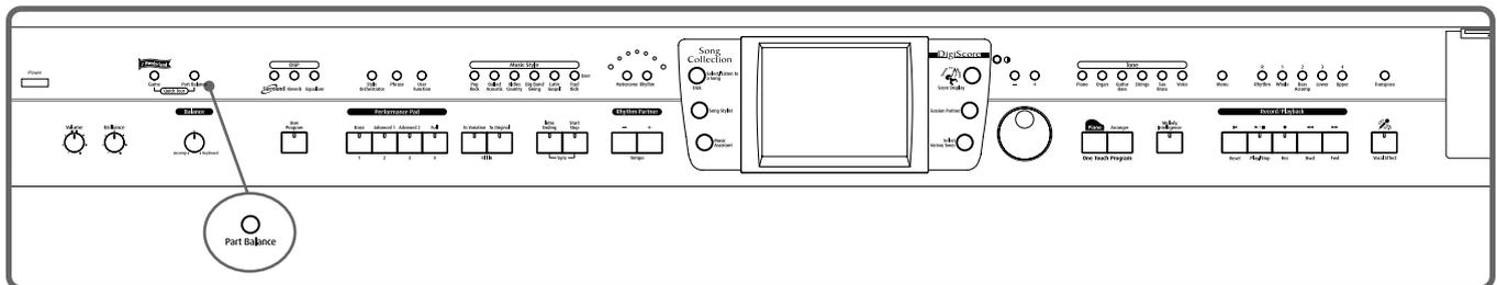
1. Press the [Part Balance] button and watch the indicator light up.
