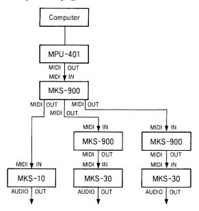
The MKS-900's are assigned to the sound modules which are to be driven by the computer. Set the Channel Selector of each MKS-900 to the appropriate Channel number that belongs to the connected sound module. Now, the performance of each sound module can be respectively glasped on the MKS-900.
