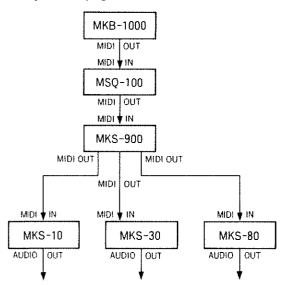
In this setup, a sequencer is used, and several MIDI channels are sent to the MKS-900. Set the Filter Switch to OFF and the Channel Selector Switch to the MIDI Channel number you like. The part of each instrument can be visually glasped without affecting the performance. When the Filter Switch is set to ON, only the sound of the selected Channel will be heard, therefore you can easily tell which synthesizer is played, on which channel.
