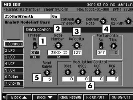
These are parameters related to overall control of the synthesizer.
