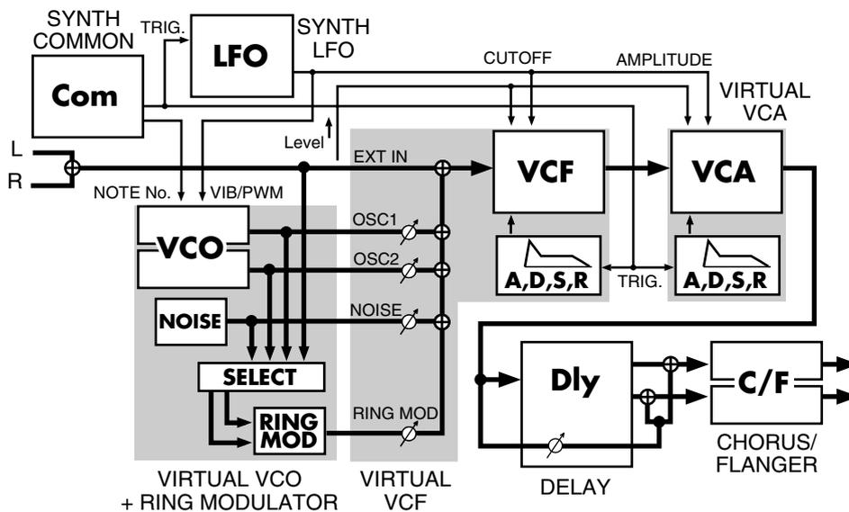
By selecting Analog Modeling Bass, you can use the MV-8000's effect section as a monophonic synthesizer. You can control note-on/off and pitch in several ways.
