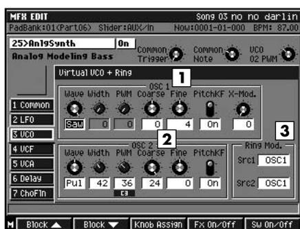
This reproduces the VCO (Voltage Controlled Oscillator) virtually. It comprises two oscillators, OSC1 and OSC2, a noise generator, and ring modulator. Settings include those for the waveforms that are the basis of synthesizer sounds and pitch settings for the two oscillators.
