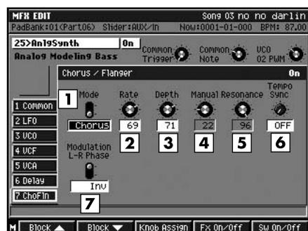
This effect can select either a chorus effect, which adds spaciousness and a wavering effect to the sound, or a flanger effect, which adds a metallic undulation (rising and falling sound).
