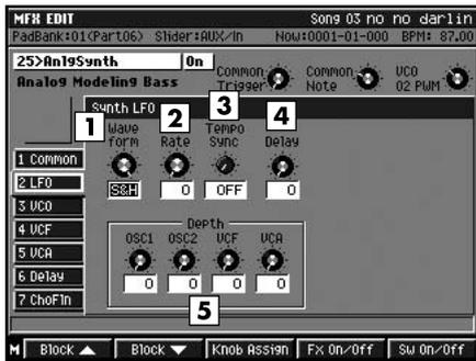
The LFO is the oscillator that creates a swelling sound. By greatly increasing the values for parameters such as VCO vibrato, PWM depth, and LFO depth (explained below), you can get various kinds of vibrating sounds (periodic, cyclical changes) in tone and pitch.
