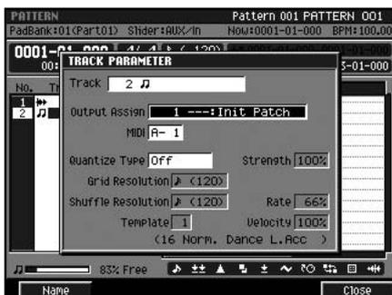
4. While using the pads to audition the sound, change the Output Assign setting so that you can hear the desired part.
