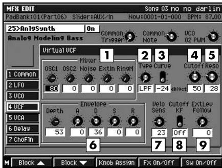
This reproduces, virtually, the VCF (Voltage Controlled Filter). The sounds from the VCO or input from external sources are processed with a filter that moves the cutoff frequency as needed, and creates brightness (or hardness) in the tone and changes in tone brightness over time. There is a mixer to set the input level from each of the sound generators at the input section of the VCF.
