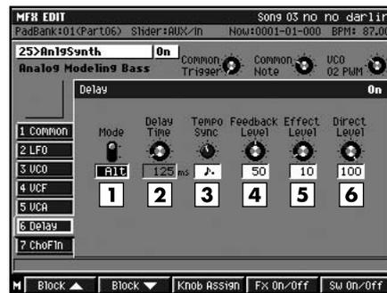
This digital delay can be switched between monaural and alternate modes (left and right channels mutually). The maximum delay of 2400 msec (2.4 seconds) provides long echoes, fat, or thick sounds.
