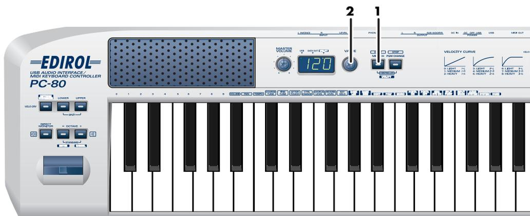
Make sure that the PC-80's **SOFTWARE SYNTHESIZER** button is not lit. If you're in Controller mode (p. 67), switch to Play mode.
