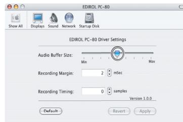
Latency is the time delay from when the software plays back audio data until the sound is actually heard from an audio device such as the PC-80.
