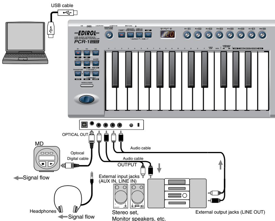
\* To prevent malfunction and/or damage to speakers or other devices, always turn down the volume, and turn off the power on all devices before making any connections.
