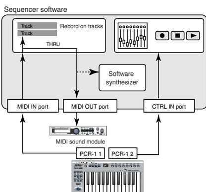
The output destination of the MIDI messages transmitted when you operate the PCR-1’s knobs, and buttons can be specified separately for each controller. (**Assign MIDI messages (EDIT)** (p. 61))
