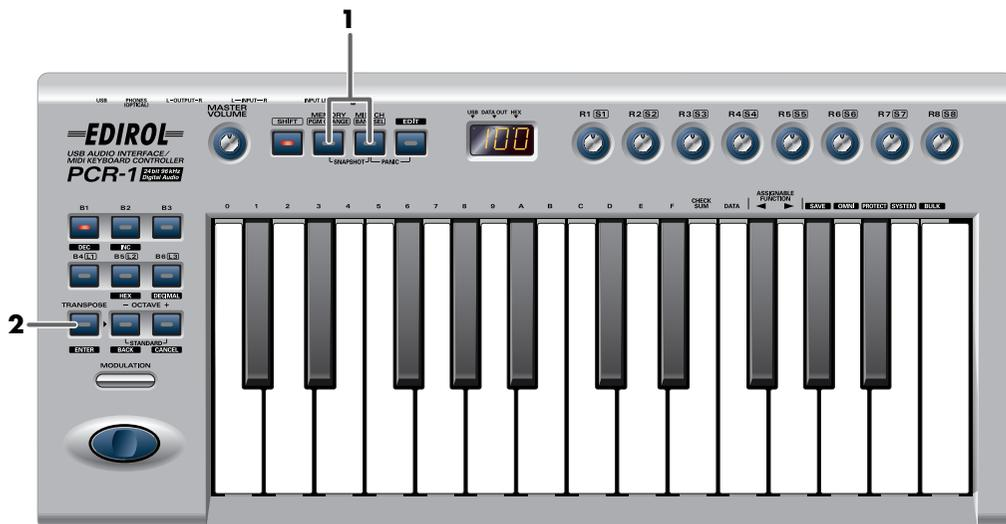
**1** Simultaneously press the [MEMORY] button and the [MIDI CH] button.
