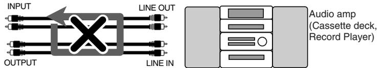
If the PCR-1 is connected as shown above to a device that outputs (“thru-s”) the input audio (such as a cassette player that is in recording mode), turning on the Input monitor switch will cause the sound to loop between the PCR-1 and the other device, causing oscillation and producing an unexpectedly high volume. Be aware that such connections may cause the system to malfunction, or your speakers to be damaged.
