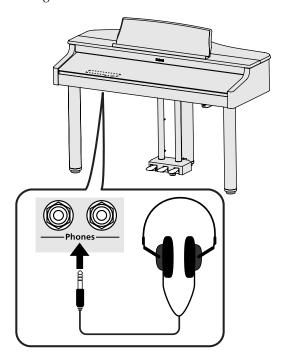
1. Plug the headphones into a Phones jack located in the jack panel on the RG-1's bottom left panel.
