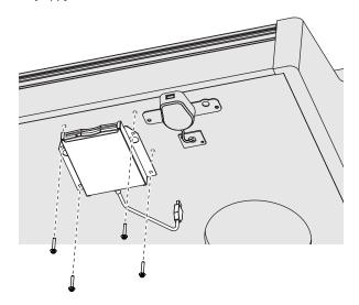
**2.** Connect the USB cable included with the floppy disk drive to the External memory connector on the RG-1.
