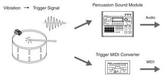
The RT-10K Kick Trigger and RT-10T tom trigger support head triggering. The RT-10S Snare Trigger supports separate head/rim dual triggering.
