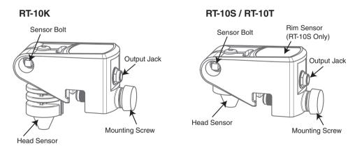
\* Do not place excessive pressure on the sensor and do not leave it mounted for extended periods (for example when not in use) or with pressure exerted from an angle. Following these instructions will guarantee efficient triggering and prevent damage.
