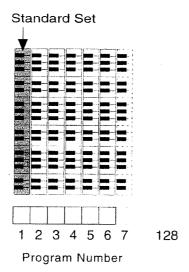
\* Although Program Numbers range from 1 to 128, there are nowhere near that many different Drum Sets on the SC-55ST. If you try to select a Drum Set that doesn't exist, you'll get the previously selected Drum Set sounds. Check the Drum set list (P. 25) to make sure that the Program Change message you are sending cor-
