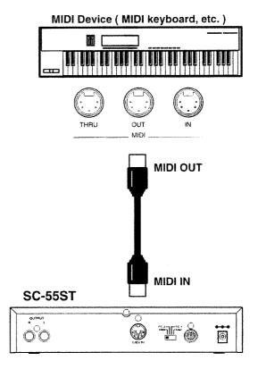
In addition, if you already have a MIDI interface, you can connect the SC-55ST directly to it. When connected in this way, the SC-55ST can be operated just like any other MIDI sound module.
