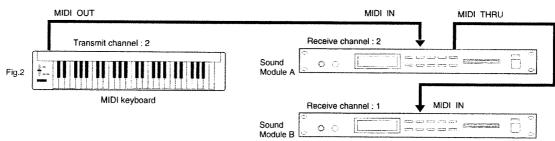
SC-55ST can receive a total of 16 channels simultaneously. By using 16 channels you can play ensembles of 16 Parts. Sound sources such as the SC-55ST which are able to simultaneously play many parts are called multi-timbral sound modules. Timbre is a word meaning sound.
