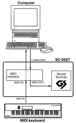
When connected to a computer by means of a COMPUT-ER Cable, the MIDI IN connector on the SC-55ST becomes the computer's (MIDI interface's) MIDI IN. For this reason, you will not be able to play the SC-55ST's sounds if left this way. In order to have a MIDI keyboard play the SC-55ST's sounds, you must turn on the Soft Thru function within your MIDI application. (Soft Thru is a feature which will cause all MIDI messages that arrive at MIDI IN to be retransmitted from MIDI OUT.)
