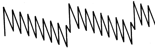
Fig. 1-6 VCO sync wave forms for the sawtooth wave.
