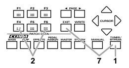
1. Press [TUNER/BYPASS]. The Tuner function will be turned on.
