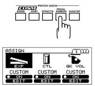
2. Press [F2] (ON/OFF) to switch the CTL pedal function on/off.
