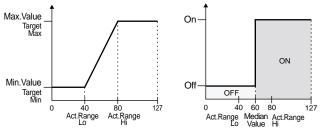
\* If you are using an on/off type controller such as a foot switch as the source, please leave this at the "LO:0" and "HI:127" settings. With other settings, the value may fail to change.
