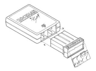
1. Remove the ROCKMAN battery door and batteries and insert the ROCKADAPTOR into the empty battery compartment. Match the front and rear labels of the ROCKADAPTOR with the ROCKMAN.
