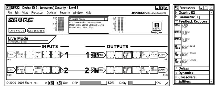
The primary interface for the DFR22 is a Windows-based software program that mimics the functional block diagrams used in sound system design. Unlike many other DSP products that constrict freedom with preset templates, the processing blocks in the DFR22 can be applied in any order, to any input or output. Processing blocks can be copied and pasted to duplicate processors across multiple channels. They can also be linked for more efficient stereo or global control.
