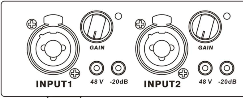
2 x combo (XLR & TRS) connectors are provided as channel inputs. Connect the source audio material you would like to pre-amplify and/or convert to a digital stream to these connections.
