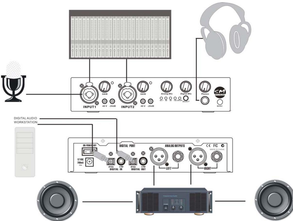
The ADDA 192-S's replaces sub-standard converters and allows your all-important analog connections and conversion to operate away from any possible electrical interference that can be inherent in your computer chassis.
