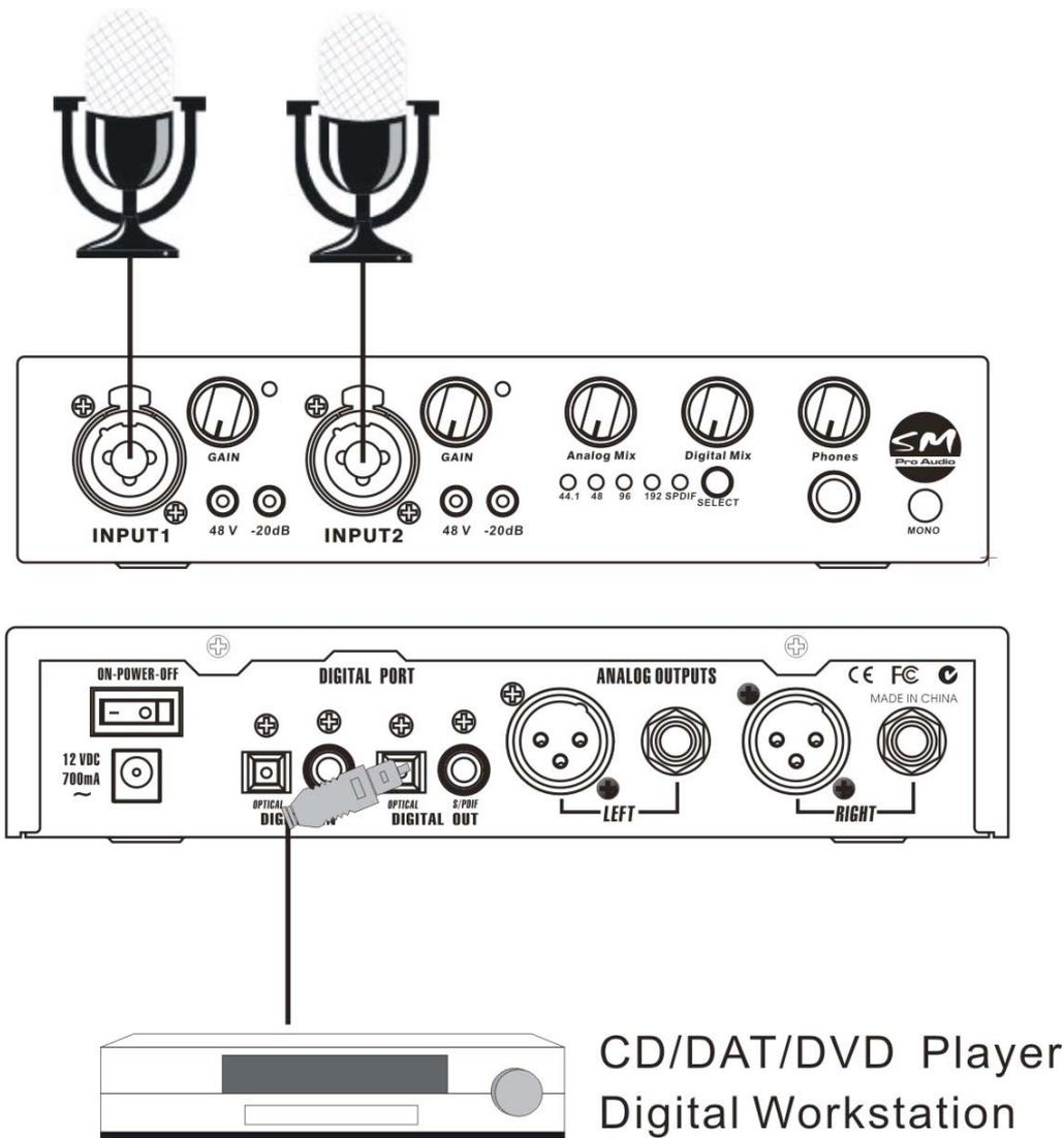
Mobile portable DAT machines, stand-alone CD/DVD recorders, etc. are often the perfect recording medium when out on the road or in the field. The only problem is that they don't feature any built in microphone pre-amplifiers!
