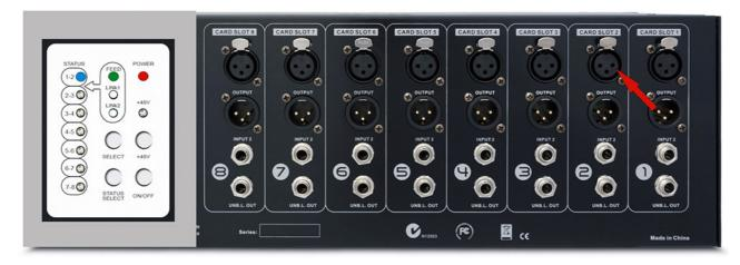
input into module 1 gets processed then outputs to module 2.
