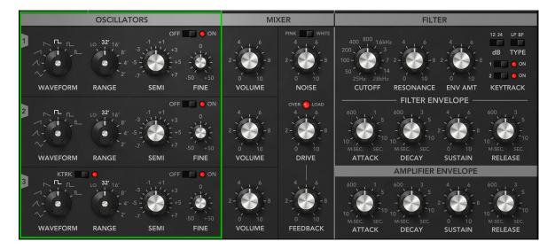
The Legend uses three oscillators as the core of its synthesis, which produce periodic pitched tones. All oscillators share the same sound parameters explained below.
