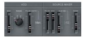
The *Range* parameter switches the octave of the *VCO* (16'/8'/4'/2'). The *Mod* parameter adjusts the modulation intensity of the *LFO*.
