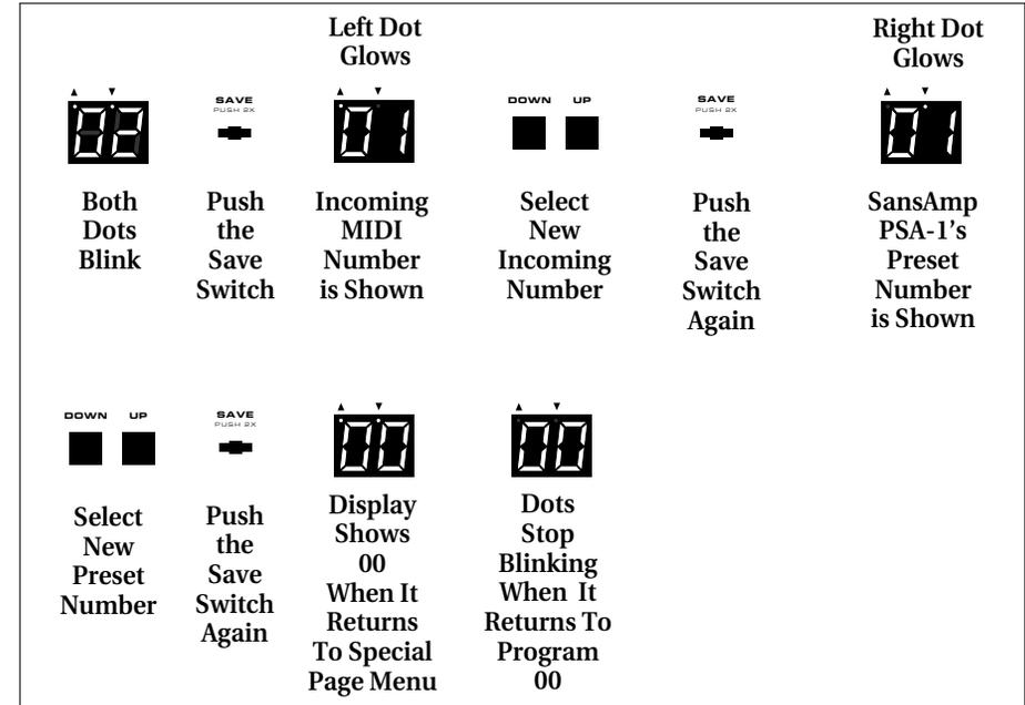
display is showing the number of the incoming program. To change that number, use the **Up** and **Down** switches to select a new number. Now push the **Save** button and the right dot
