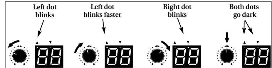
the dot blinks faster. If you turn the knob past the preset point, the right dot will first blink fast and then slow as you turn farther clockwise away from the preset point. When you reach the preset point, both dots stop blinking and go dark.
