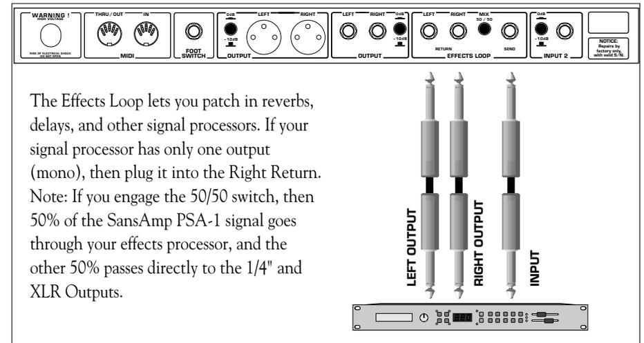
The Effects Loop lets you patch in reverbs, delays, and other signal processors. If your signal processor has only one output (mono), then plug it into the Right Return. Note: If you engage the 50/50 switch, then 50% of the SansAmp PSA-1 signal goes through your effects processor, and the other 50% passes directly to the 1/4" and XLR Outputs.
