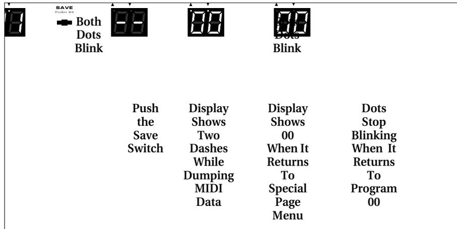
dashes for approximately 10 seconds, and then 00, meaning that it has completed the dump. After doing the dump, it returns to the Special Page function menu. You may now choose either a new Special Page function, or press **Save** again to exit. If you don't make a choice in about 15 seconds, the display reverts to 00 without the dots blinking, indicating that the SansAmp PSA-1 is in Program 00, bypass.
