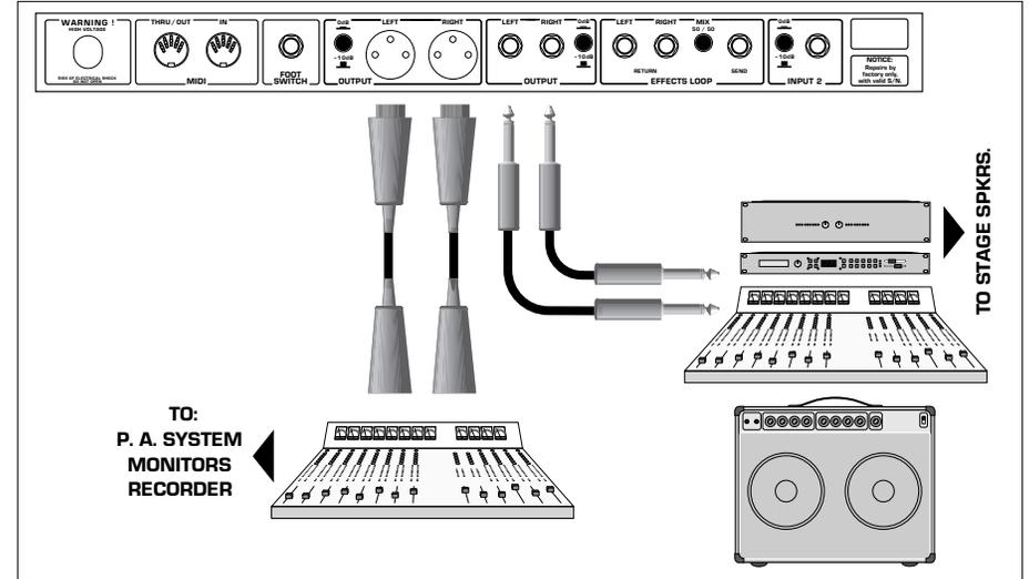
The SansAmp PSA-1 has dual 1/4" unbalanced and XLR balanced Outputs for interfacing with all types of gear. XLR Outputs provide a signal for driving pro gear, including P.A. systems, mixers, signal processors. 1/4" Outputs are ideal for feeding most mixers, signal processors, and instrument amplifiers. Each set can be used simultaneously and independently.
