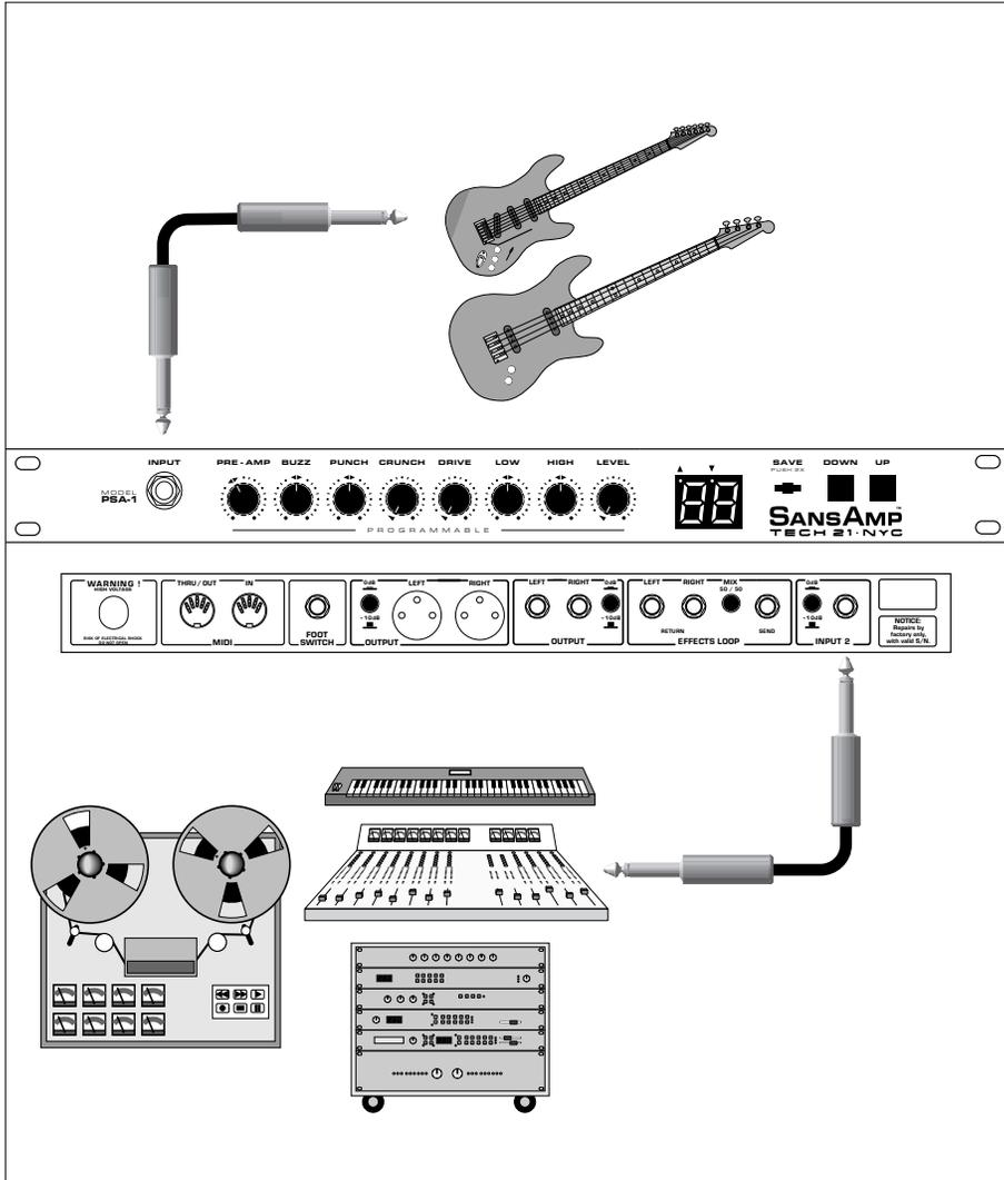
The front-panel Input jack is designed to accept signals from guitars, basses, keyboards, etc. You can set up your SansAmp PSA-1 as a permanent part of a rack or patch-bay setup, with its usual input source plugged into the rear-panel jack. Then, if you want to plug straight into the SansAmp PSA-1, use the front-panel Input, which overrides the rear-panel Input 2.
