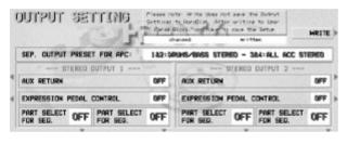
Basically the 4 separate audio outputs are 2 selectable stereo lines direct from the tone generator.
