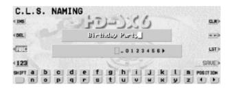
Write the name of the script file in the way as naming on the KN6000/6500. Up to 16 characters are allowed.
