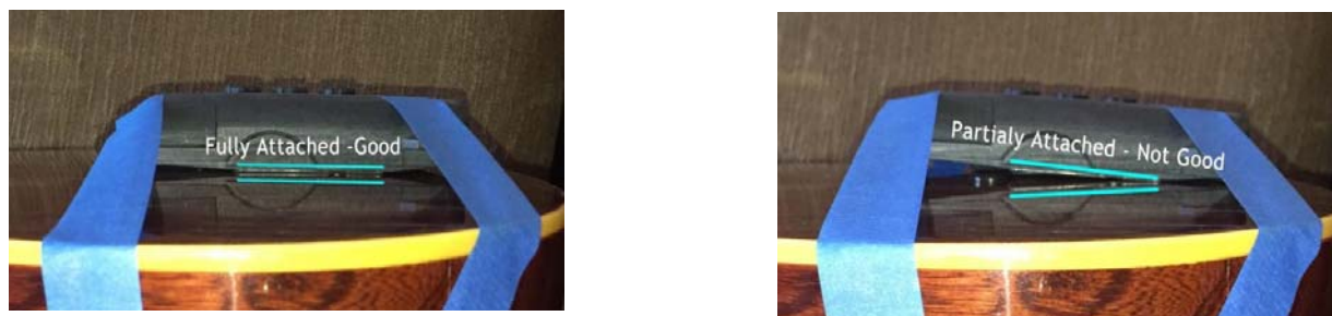
Figure 2-4 ToneWoodAmp taped properly (left) and incorrectly (right)
