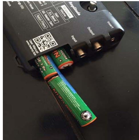
Figure B-2 The tape is nested between the two top batteries
