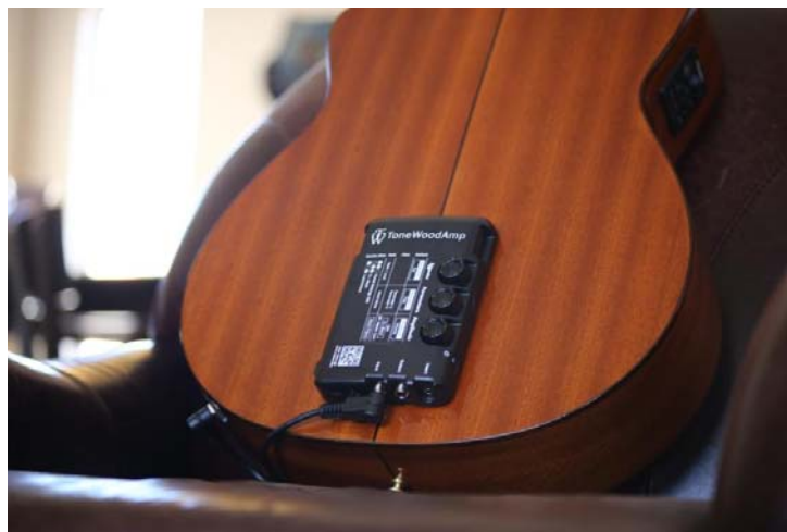
Figure 2-6 ToneWoodAmp mounted on back of guitar
