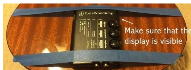
Figure 2-3 ToneWoodAmp taped in position for testing
