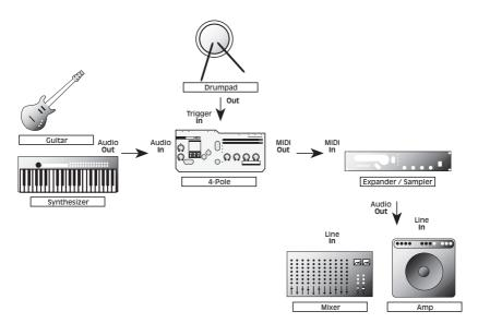
You can trigger any signal you have patched into the <Audio In> jack. You can also connect a MIDI sound generator to the <MIDI Out> jack and play its sounds via your drumpad. You will probably have to assign the MIDI channel and the note number (Section 5.6).
