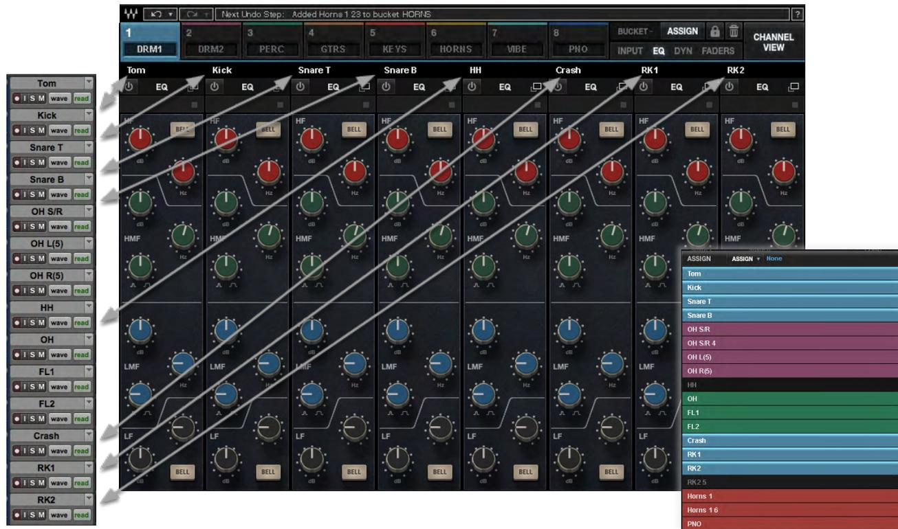
In this example, eight tracks in the host DAW are assigned to one CLA MixHub bucket. Note the corresponding track names. With supported hosts, track names will automatically copy to the MixHub assignment menu. If not, rename the tracks from within MixHub. To the right is the Track Assign list used to add tracks to the bucket. Track assignment does not need to be sequential. Tracks in a bucket can be mono or stereo and these can be mixed together in one bucket.
