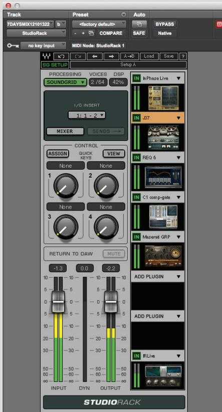
Add a DSP server to a Pro Tools HD/HDX or HD Native system to move processing from the Local CPU. This greatly increases plugins performance. Audio steaming to the server through DLI/DLS is controlled by the StudioRack plugin.
