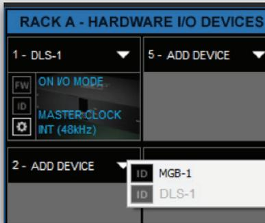
To add another SoundGrid device, click on the arrow in an empty rack slot. From the list of available devices, choose the one that you want to add, in this case, a DiGiGrid MGB coaxial MADl interface. In this image the DLS is grayed out, and therefore unavailable, since it's already claimed (in this case, by you).
