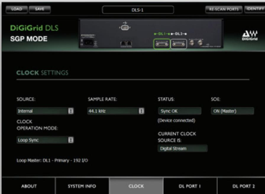
Use the **Clock Control** page to adjust clock settings and monitor the clock status of each connected device.
