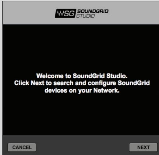
If the Wizard cannot locate the requested SoundGrid network devices, this means the devices might be off or not connected properly. In such a case the Wizard will allow you to rescan the network or work as a Driver node slaved to another system. For more information please refer the SoundGrid Studio User Guide.
