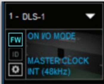
Click on the FW button to launch the Updater. This will initiate a scan of the hardware and then offer options. Do not disconnect the device or turn off the computer until you see "Done."
