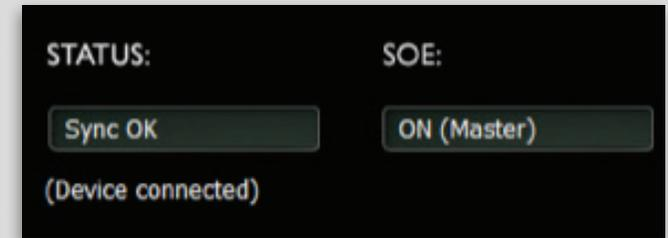
Blue text on the device icon indicates that the DLS is the SoE clock master. The SoE window on the DLS control panel indicates that the device is locked to SoE and is the master.
