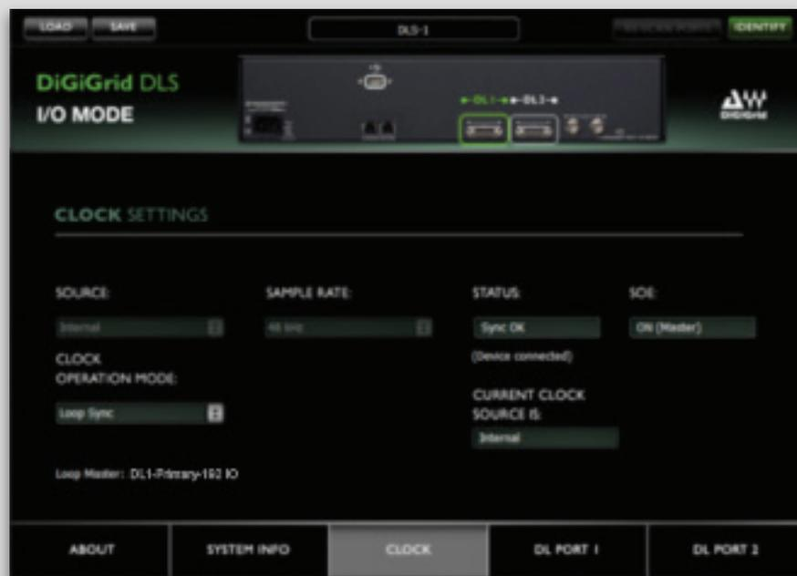
These devices are now locked to each other: one Loop Sync master (192 I/O) and Loop Sync slave (DLS, appearing to Pro Tools as “192 Digital I/O #1”). You can verify clock settings in the DLS control panel. In this example, the DLS is locked to the 192 via Loop Sync and its status is “OK.”
