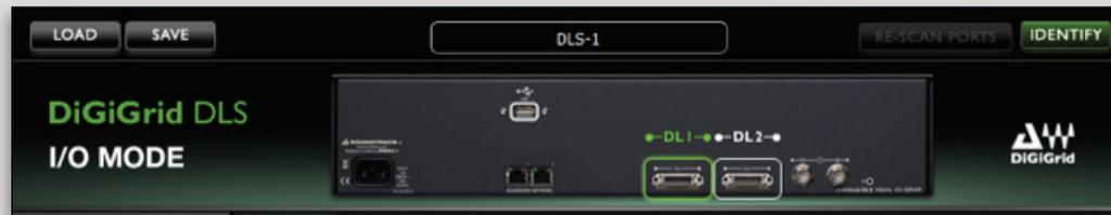
At the top of each Control page is an identification and management banner that indicates the ports connected to active devices. This page is also used to load and save device presets, rescan ports and update clock status, and identify the hardware device.
